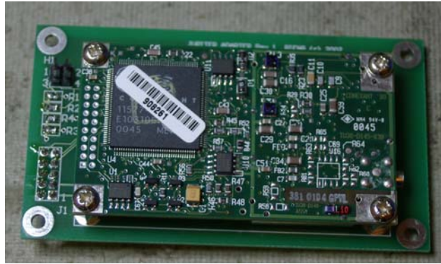
Figure 5 - Adapter Board with GPS Unit
