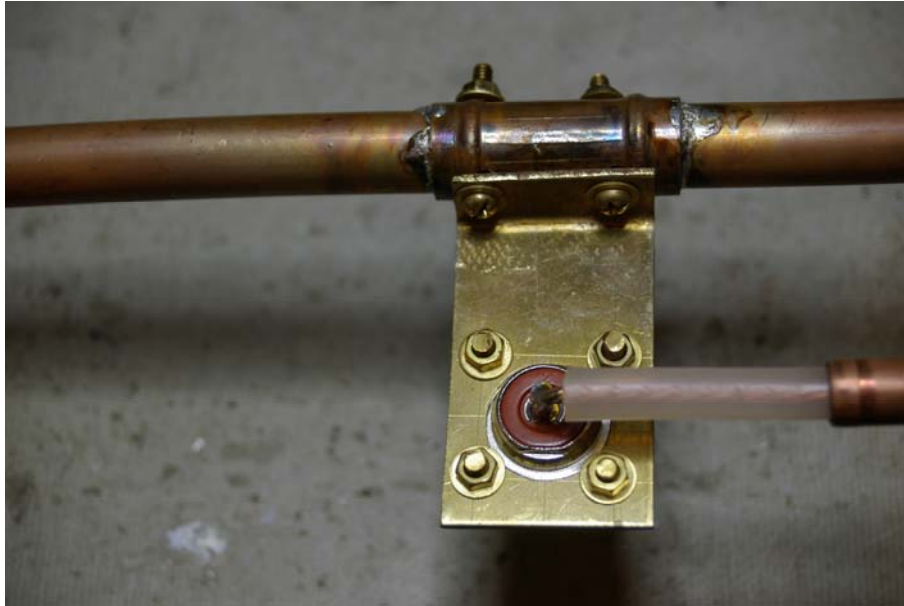
Figure 6 - Securing the Connector
